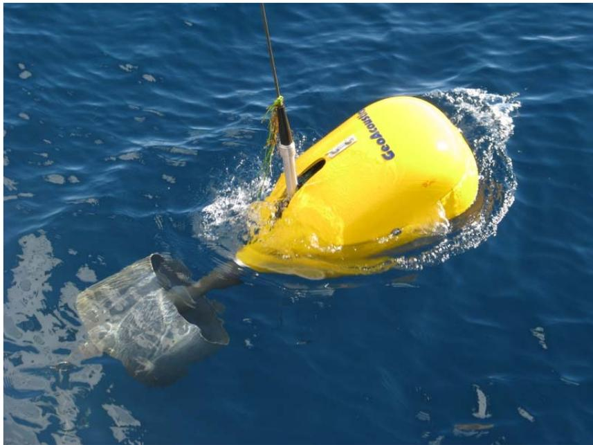
Fig. 3.7. Transducer tow of GeoPulse Sub-bottom Profiler system.
