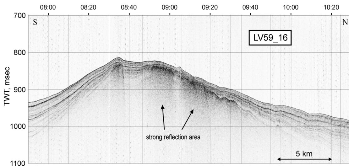
Fig. 3.18. Example of strong reflector area that is probably connected with gas-bearing stratum in the Study Area 4-1. See profile location in Fig. 3.12.
