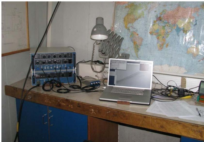
Fig. 3.8. Registration complex of GeoPulse Sub-bottom Profiler system consisting of control box (generator, amplifier and filter) and Macintosh PC control.
