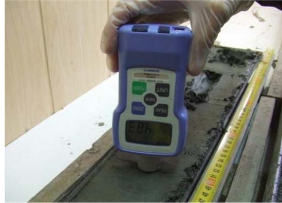
Fig. 4.4. Cone penetration test
