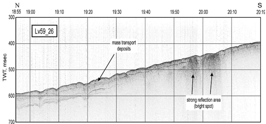
Fig. 3.17. Example of strong reflector area connected to gas expulsion. Many gas flares were detected inside this area. Left side of the profile shows weakly deformed sediment. It is suggested that deformation has occurred due to creep process. See profile location in Fig. 3.10.
