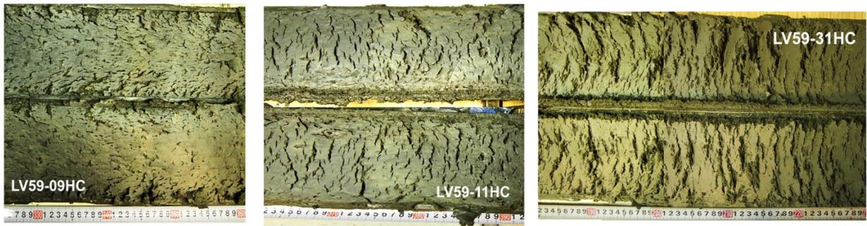
Fig. 4.9. Types of gas-saturated sediments.
