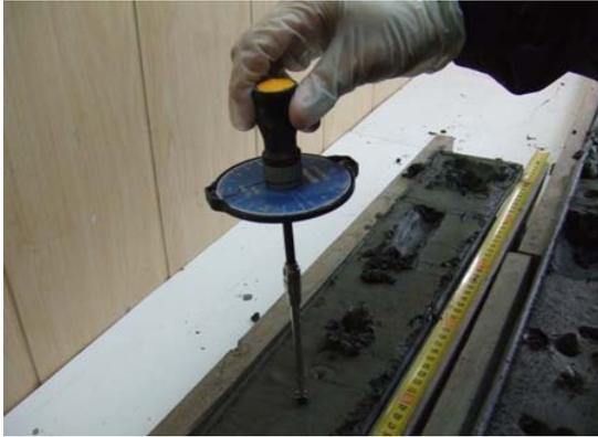
Fig. 4.3. Vane shear test
