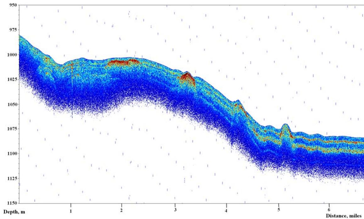
Fig. 3.26. Example echogram subbottom structure at a frequency of 12 kHz.
