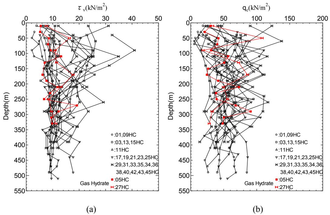
Fig. 4.5. Typical onboard test results; (a) vane shear test, (b) cone penetration test
