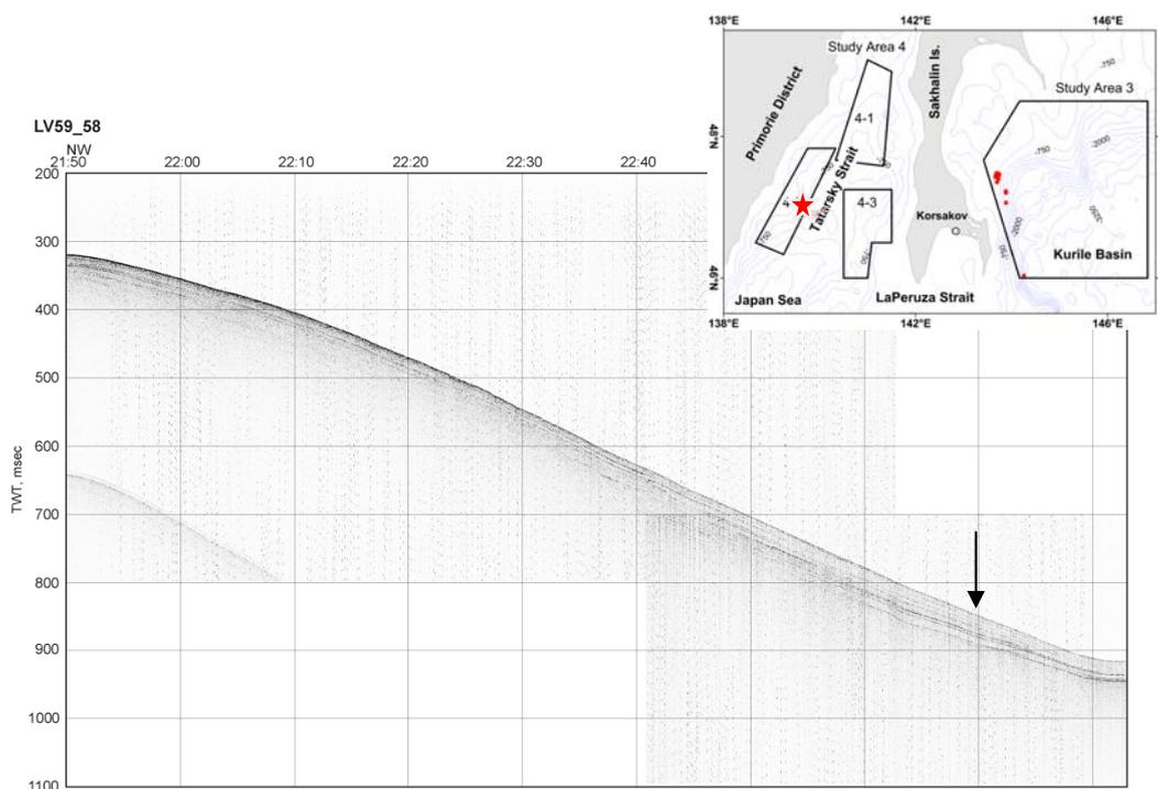
Fig. 4.11. Seismic profile LV59\_58 and the location of LV59-46HC (a black arrow in the profile and a red star in the inset) obtained in SSGH-12 cruise for paleoceanological analysis.
