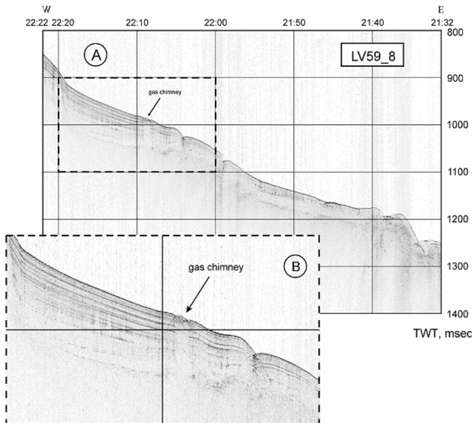
Fig. 3.16. Structure of the upper sedimentary layer on southern Sakhalin slope, seismic profile LV59\_8 (A) and part of profile LV59\_8 showing gas chimney (B). See profile location in Fig. 3.9.
