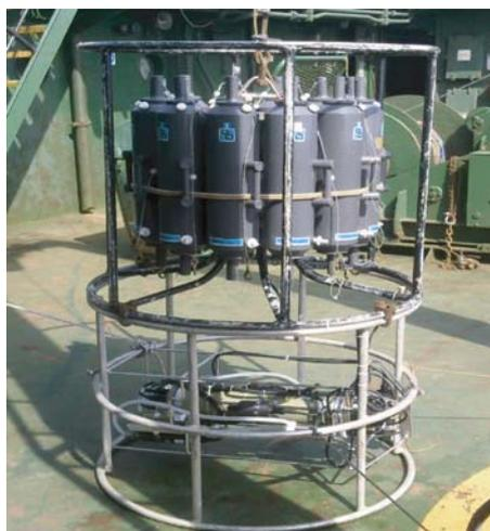
Fig. 4.13. CTD probe in the complete set with Rosette.
