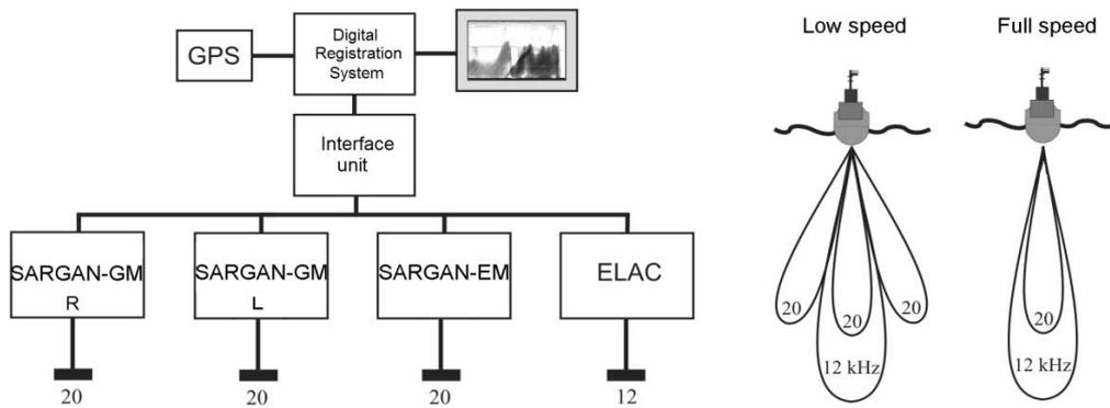
Fig. 3.21. The hydroacoustic complex block-diagram.
