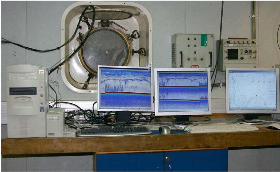
Fig. 3.20 Multichannel digital registration system
