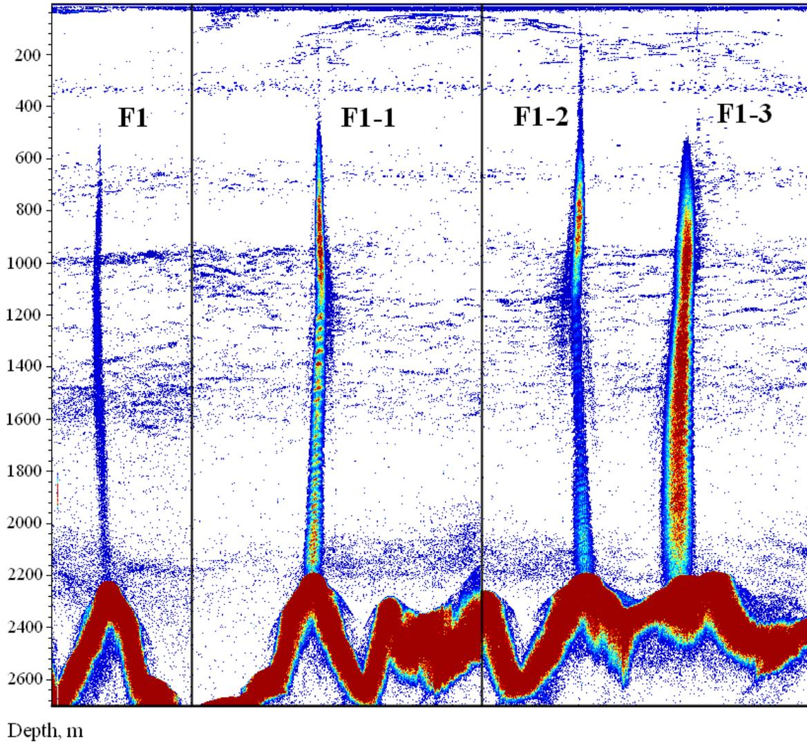
Fig. 3.24. The echogram obtained over four crossings the deepest GF F1
