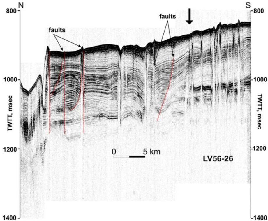
Fig. 2.1.10. Profile LV56-26 showing well-developed gas chimney structures. Arrow indicates a boundary of two areas showing different gas chimney occurrence pattern and seismic characteristics. See Fig. 2.1.2 a for location.
