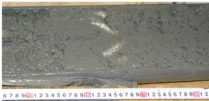
Fig. 3.3.5.6. Lenses of gas hydrates in the core LV56-03HC.
