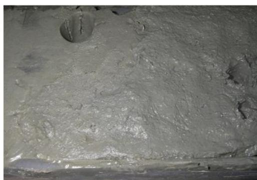
Fig. 3.3.5.7. Sinuous boundary between dense and water saturated sediments.
