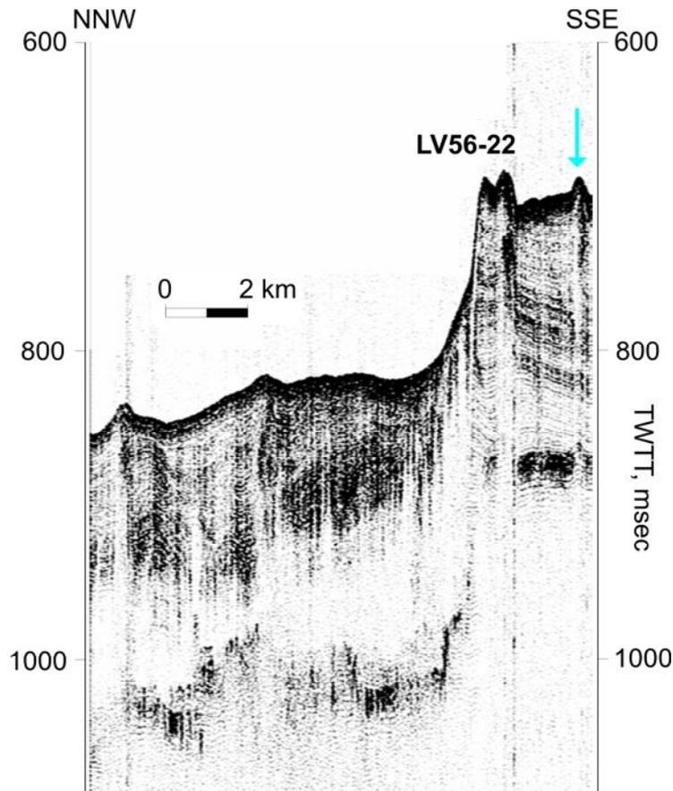
Fig. 2.1.9 Seismic profile LV56-22 showing gas chimney with gas flare marked by blue arrow. See location in Fig. 2.1.7.
