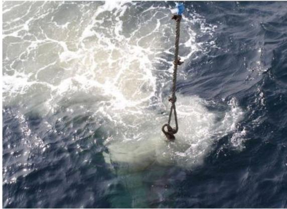
Fig. 3.3.5.3. Methane outflow during lifting of hydrocorer with sediments.
