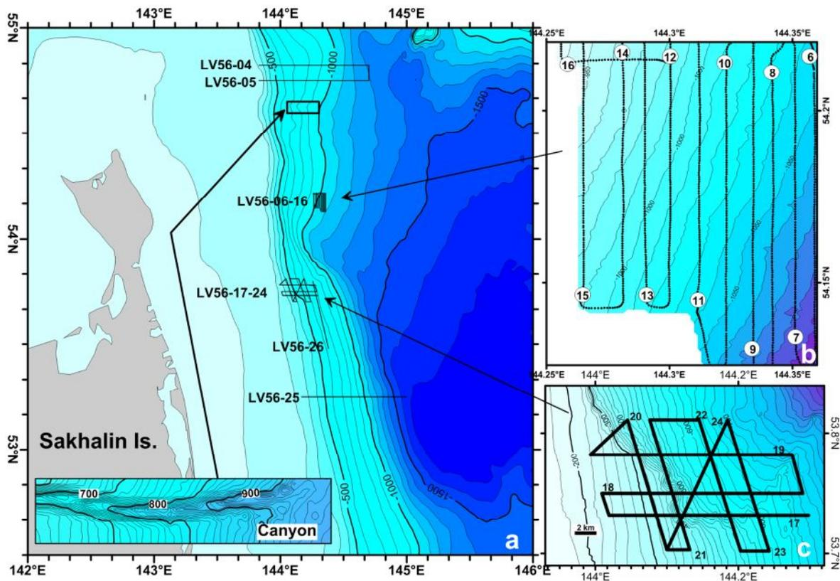
Fig. 2.1.2. Location of the seismic profiles and their number in study areas 1 (a), area of seepage field 9 (b), and Lavrentyev Fault Zone (c). Inset on Fig. 1a shows the bathymetry of the canyon, which is northern boundary of the Northern segment. Contour interval is 10 m.
