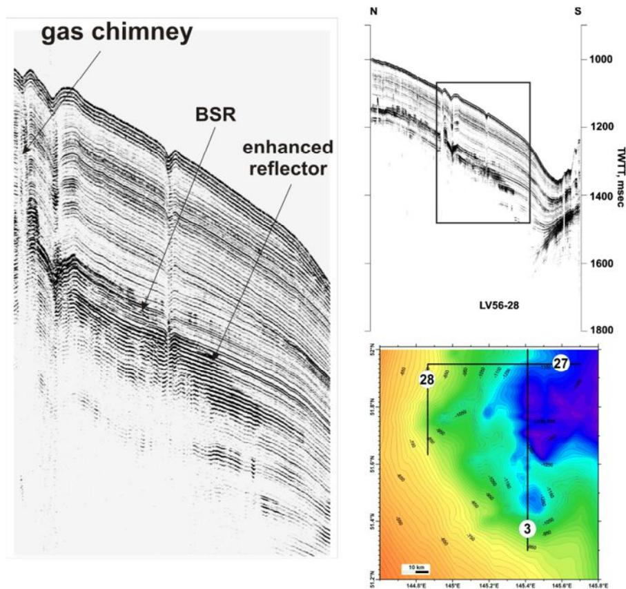
Fig. 2.1.14. BSR, enhanced reflector and gas chimneys start to appear in upper part of the slope inside Study area 2.
