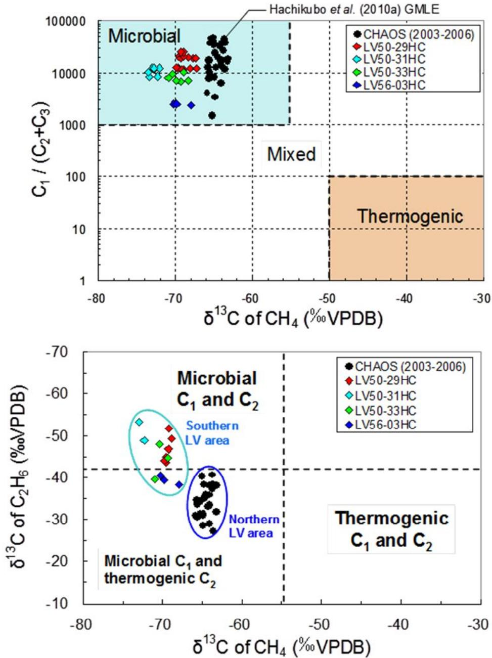
Fig. 3.3.2.1. Relation between molecular and isotopic compositions. upper:  $C_1$   $\delta^{13}C$  and the ratio  $C_1/(C_2+C_3)$ . lower:  $\delta^{13}C$  of  $C_1$  and  $C_2$ . The gas origin fields are in accordance with Bernard *et al.* (1976), Taylor *et al.* (2000), and Milkov (2005). Data of CHAOS project (2003-2006) are shown in Hachikubo *et al.* (2010a), and those of SSGH10 (LV50 cruise) are shown in Jin *et al.* (2010). The data of LV56-03HC are the new data of SSGH11.
