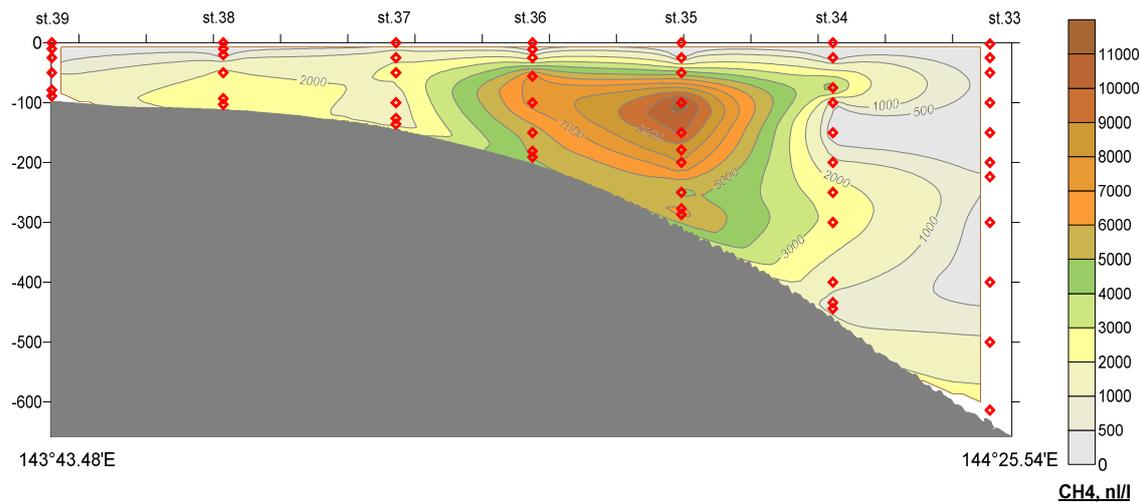
Fig. 3.4.2.2. Gas geochemical profile station LV56-33 – LV56-39 of expedition LV56, OkhotskSea that show intermediate water layer 50-250 m with great methane anomaly (10000-11000 nl/l)
