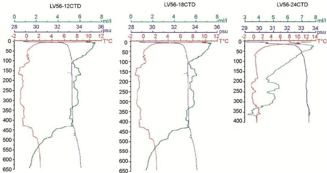
Fig. 3.4.1.6. Vertical profiles of temperature (red), salinity (dark blue) and dissolved oxygen (green) in the seaward (St. LV56-12CTD), on a slope (St. LV56-18CTD) and close to a shelf (St. LV56-24CTD).
