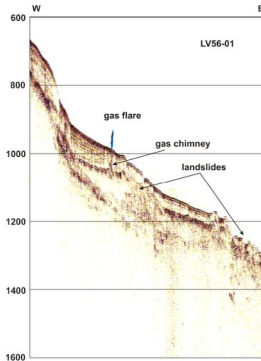
Fig. 2.1.17. Part of profile LV56-01 showing structure of the sedimentary cover across the gas flare recorded during LV56 cruise.
