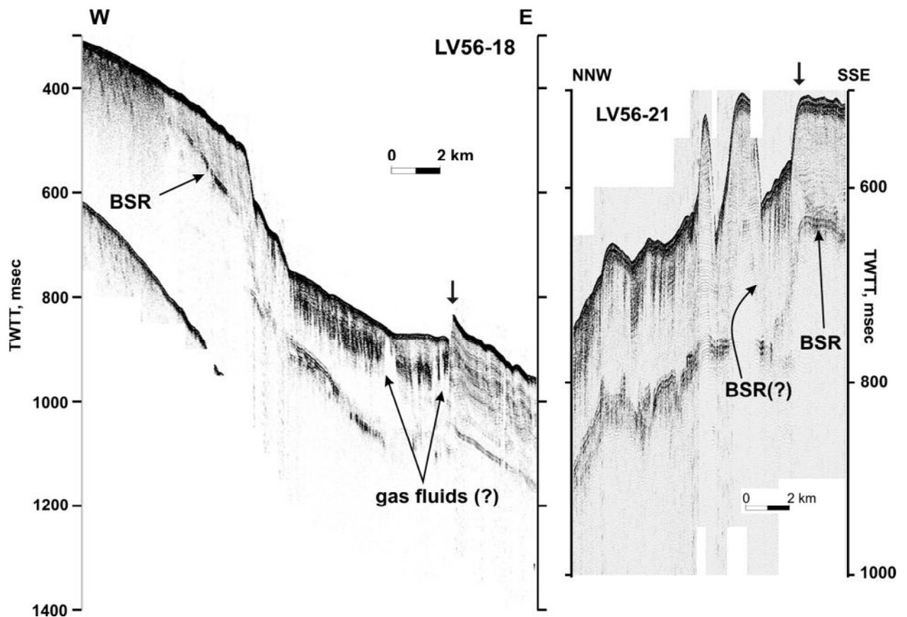
Fig. 2.1.8. Seismic profiles LV56-18 and LV56-21 showing structure of junction area between NW and NE-striking faults of LFZ. Arrows mark NE-striking fault on profile LV56-18 and WE-striking fault on profile LV56-21. See Fig. 2.1.7 for profiles location and text for additional explanation.
