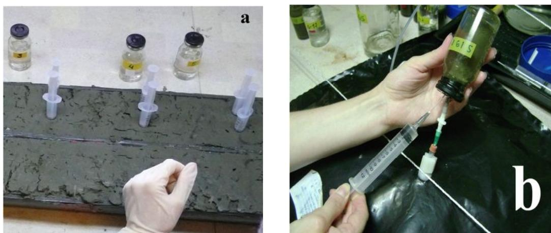
Fig. 3.4.2.1. Procedure to measure gas is using method Head Space. 1-a – choice sample of sediment from core, 1-b – to put helium in salt water with sample of sediment to analyse gas.
