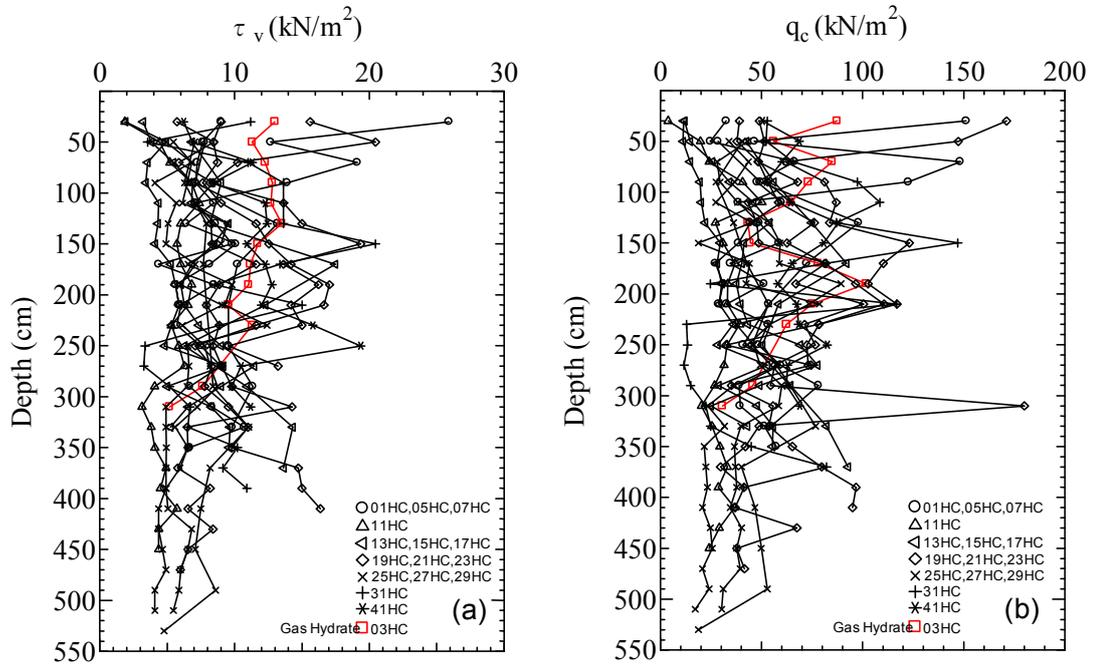
Fig. 3.3.4.1. Typical onboard test results; (a) vane shear test, (b) cone penetration test
