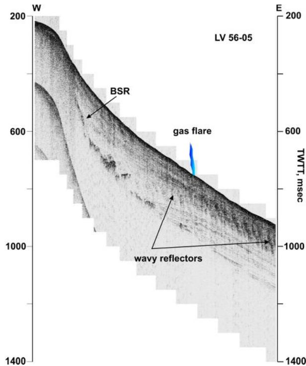
Fig. 2.1.4. Part of seismic profile LV56-05 showing location of the BSR and gas flare. See Fig. 2.1.2a for location.
