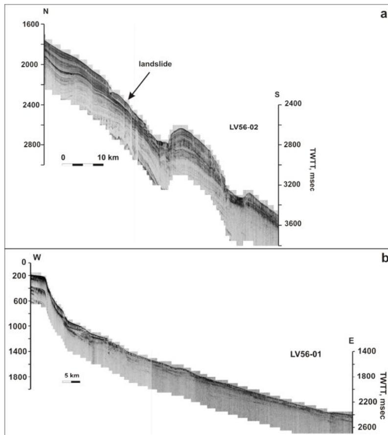
Fig. 2.1.16. Seismic profiles showing upper sediment structure for Kurile slope (a) and Aniva part of slope (b). See Fig. 2.1.3 b for profiles location.
