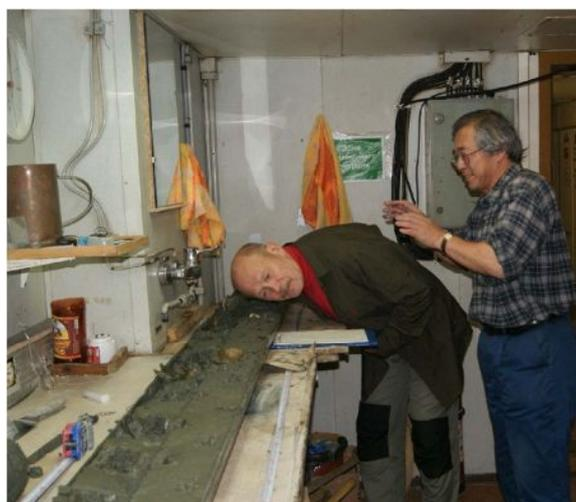
Fig. 3.3.5.8. Sediment cracking under decomposition of gas hydrates microcrystals.
