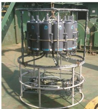
Fig. 3.4.1.2. CTD probe in the complete set with Rosette.
