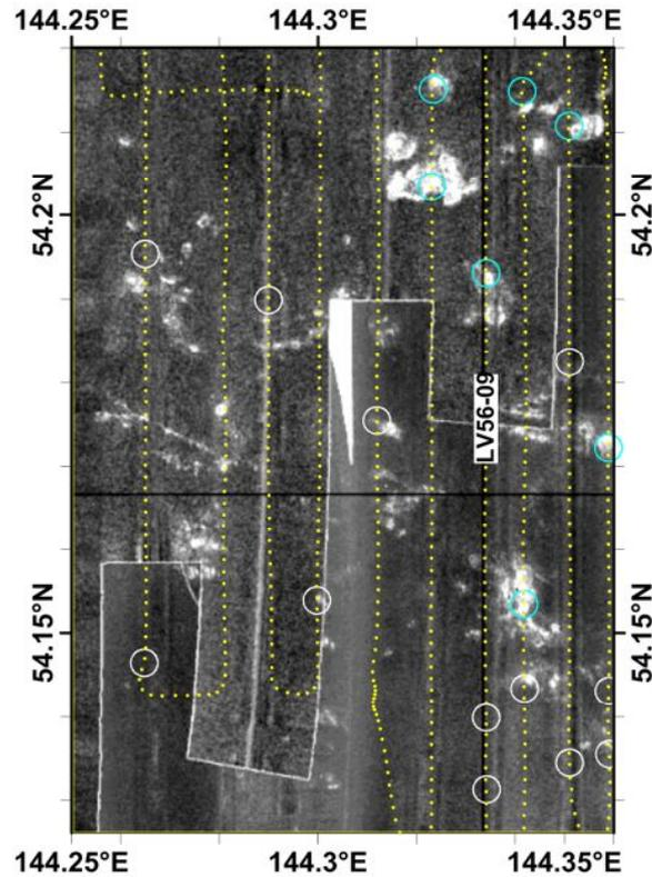
Fig. 2.1.6. Side-scan sonar image of the seepage structure field F9, location of the track lines (yellow dots) and gas chimneys. Blue open circles indicate distinct gas chimneys that reach the sea floor, white open circles mark “blind” or indistinct chimneys.
