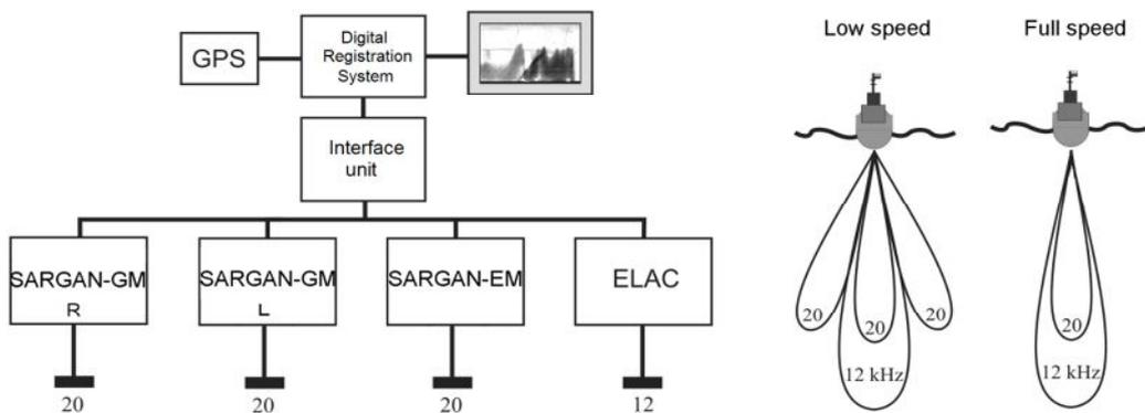
Fig. 2.2.3. The hydroacoustic complex block-diagram.
