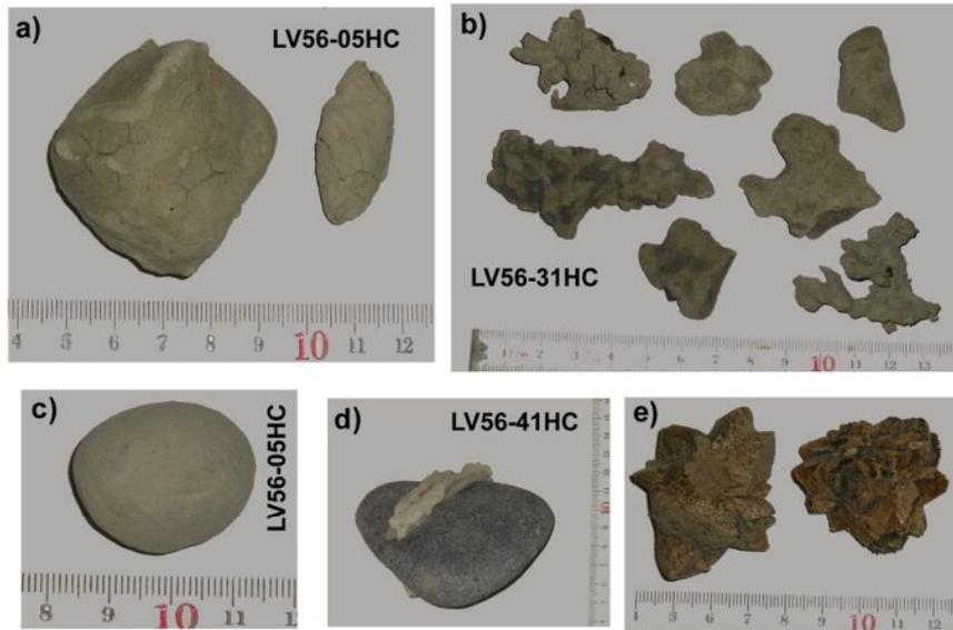
Fig. 3.3.5.4. Types of carbonate precipitates.
