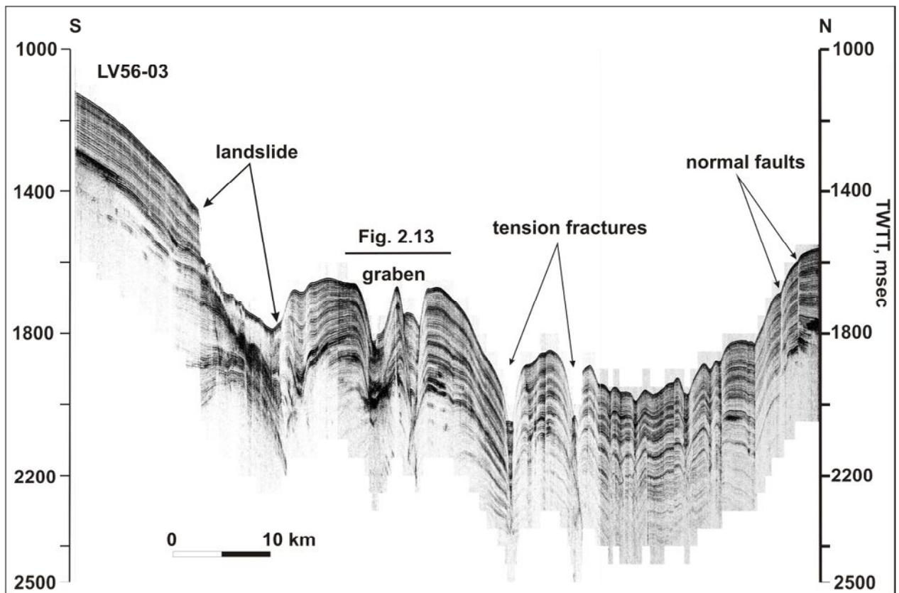
Fig. 2.1.12 Seismic profile LV56-03 across the boundary between Southern and Central segments. Numerous disjunctive dislocations have seen on this profile. See location in Fig. 2.1.3a.
