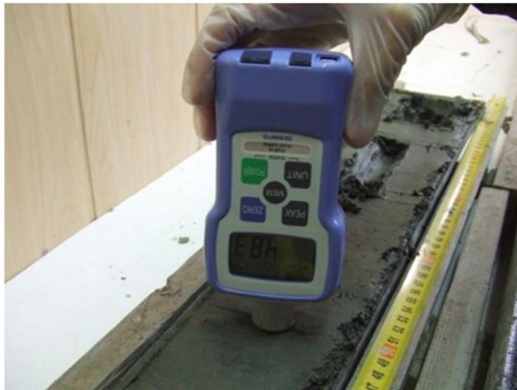
Photo 3.3.4.2. Cone penetration test
