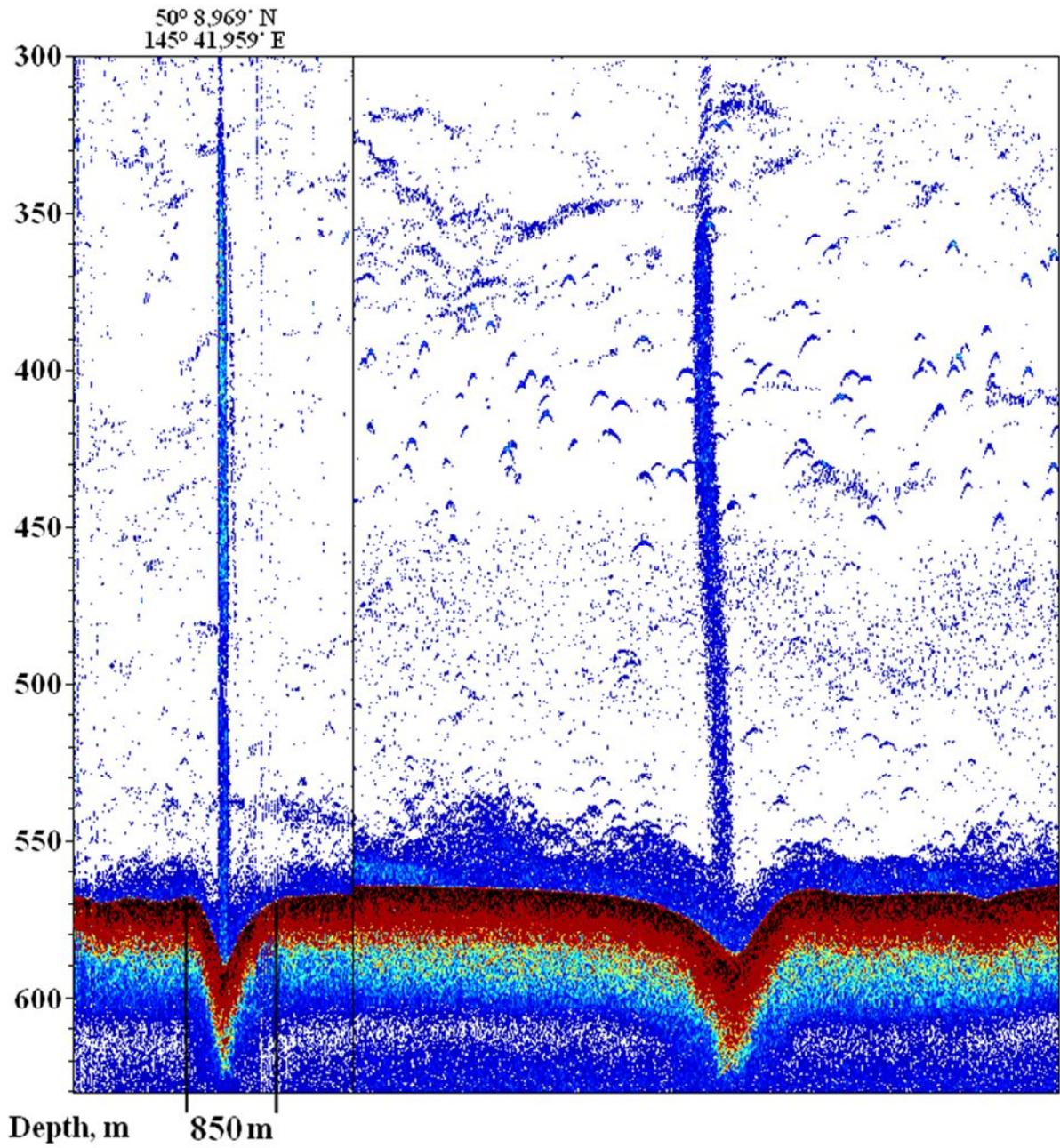
Fig. 2.2.6. The echogram GF obtained over two crossings of pockmark.
