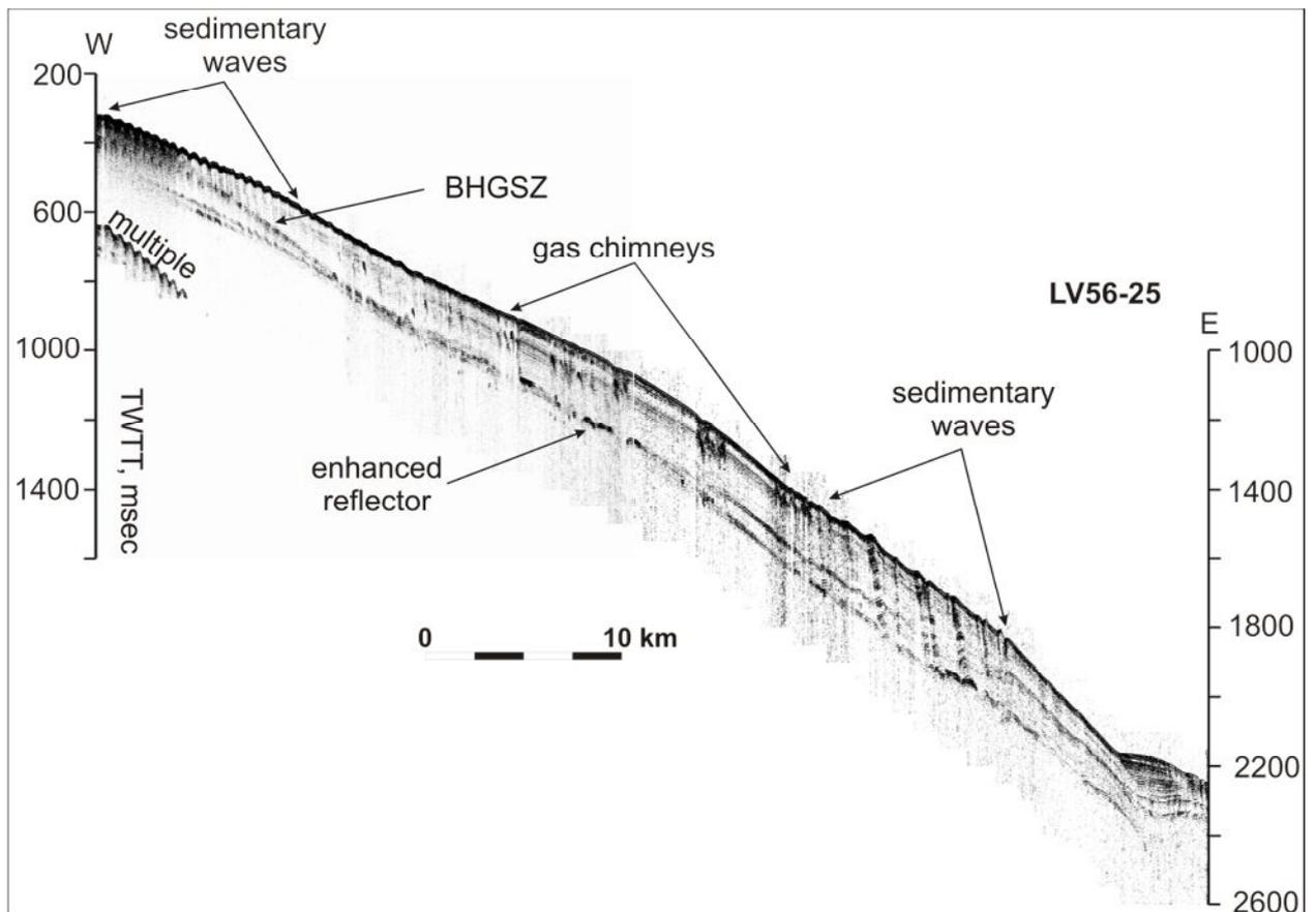
Fig. 2.1.11 Structure of the upper sedimentary cover in the southern part of study area 2. See Fig. 2.1.2a for profile location.
