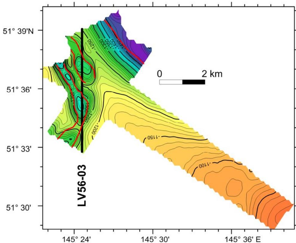
Fig. 2.1.13. Multibeam echosounder map of the Station 7 (cruise SO-178). Contour interval is 10 m. Black lines mark location of seismic profile, red lines indicate faults. Location of seismic profile crossing this map is shown in Fig.2.1.12.
